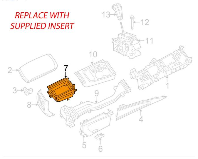
Disassemble factory center console to gain access to bin insert under armrest. Route extension harness from the T-Harness behind the radio to the location of the CD player, as pictured.
